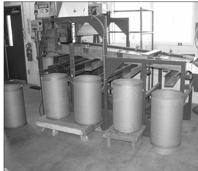
Figure 25 —Chapter 3, Seed Harvesting and Conditioning: cleaner-sizer machine has 5 screens to give 6 separations at once.
