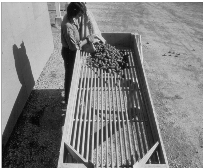
Figure 11 —Chapter 3, Seed Harvesting and Conditioning: a grading table for quick inspection and cleaning of cones or fruits (Lott and Stoleson 1967).
